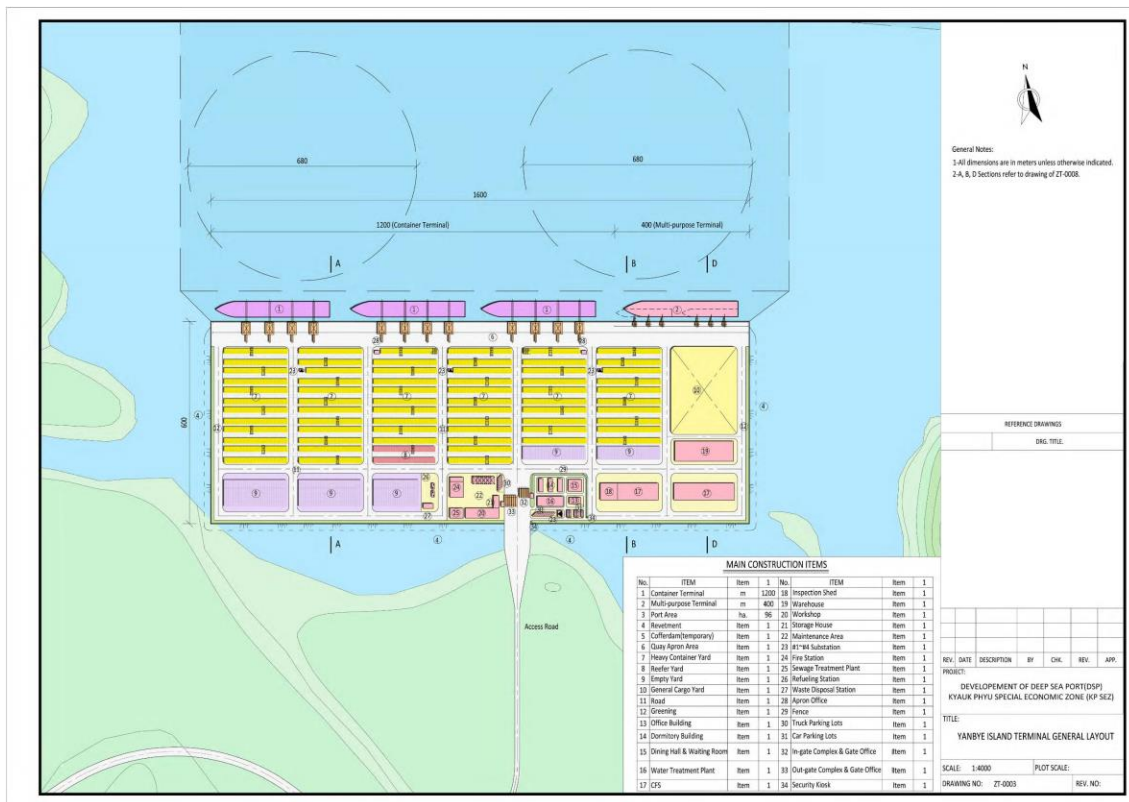
Figure 3-2: Project Layout of Yanbye Island Port Terminal of the Project (Source: CITIC)
