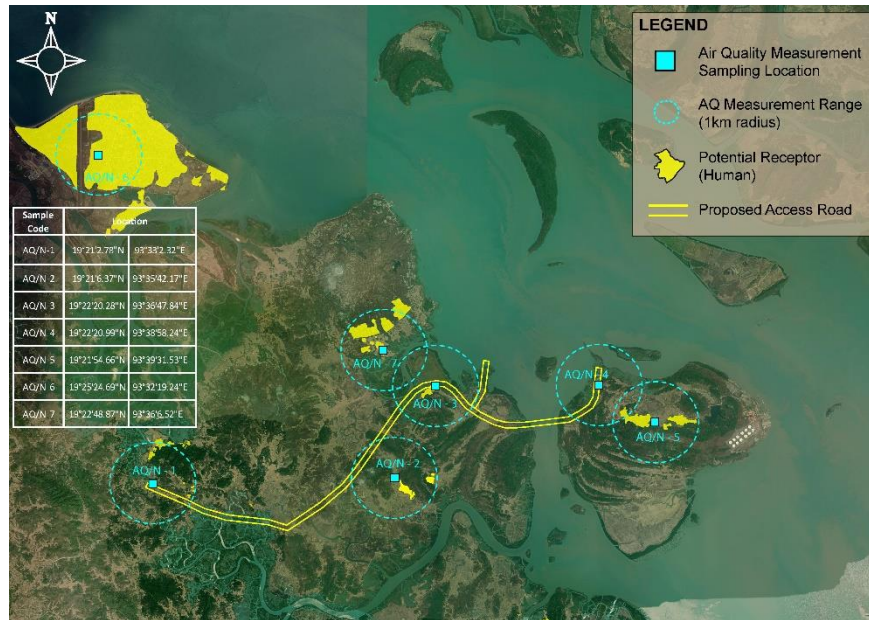
Figure ToR 3: Aerial Photo - Tentative location of Air and Noise Sample Collection Points for Baseline Environmental Ambient Air Quality Data for Access Road Development
